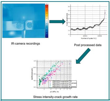
In an inventive approach, an infrared (IR) camera is employed to monitor the temperature on the rear surface of the compact tension (CT) specimen, according to ISO 15850:220(E). Simultaneously, a traveling microscope (TM) is mounted on the frontal side of the specimen to facilitate manual measurement of crack growth, as illustrated in Fig. 1.
